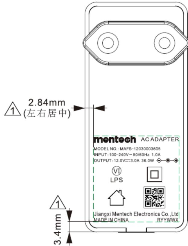
**10、STRUCTURE AND DIMENSION 结构尺寸规格**
